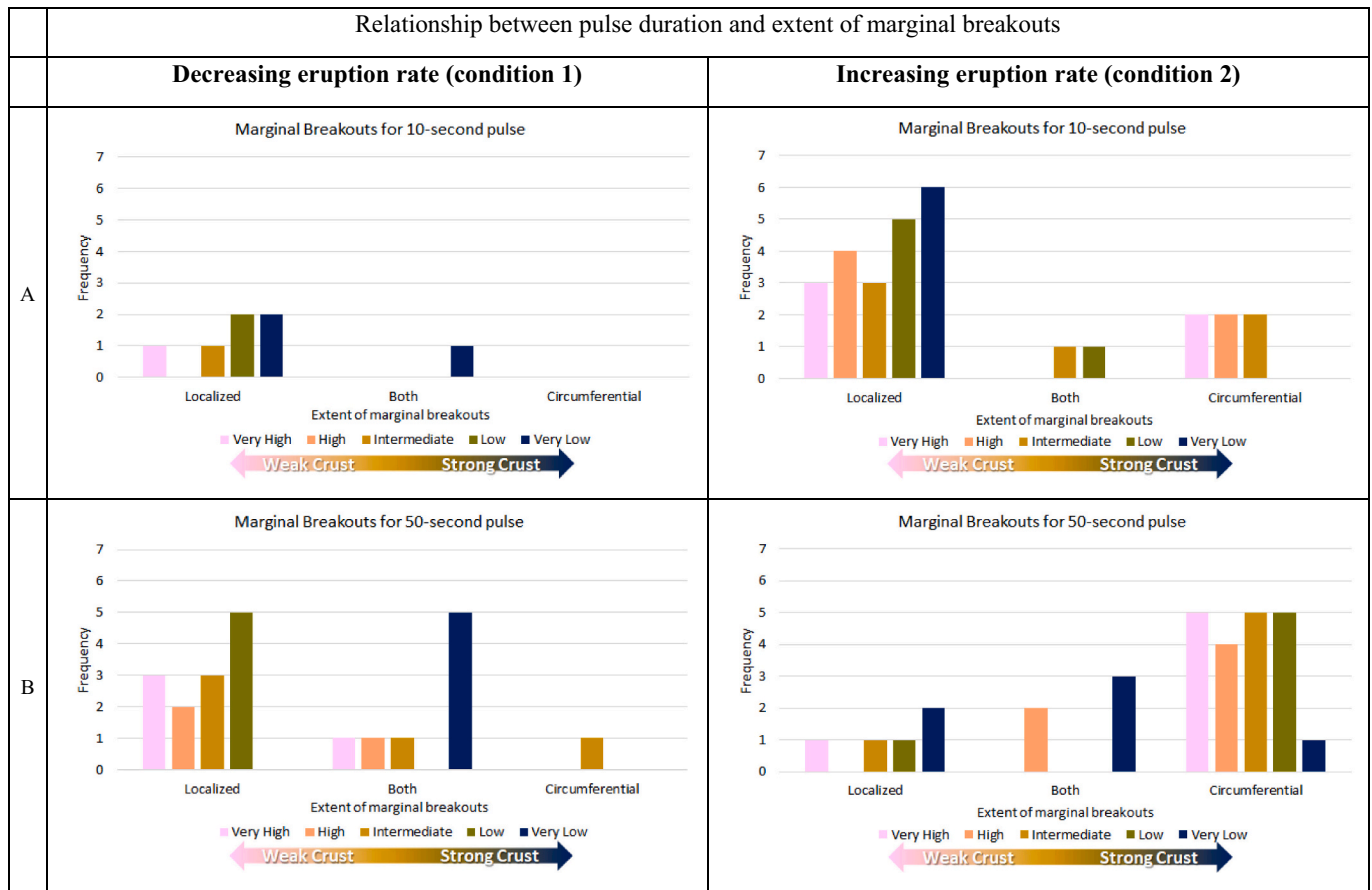
Fig. 8. The relationship between pulse duration and the extent of marginal breakouts, which contribute to flow advancement. Color bars refer to \Psi regime (from very high to very low) which also correspond to crust extent and strength. (a) For the short pulse in condition 1, marginal breakouts were rare and localized. This translates to limited flow advancement. A weak correlation on \Psi is observed. For condition 2, marginal breakouts occur frequently during the short pulse. Although most are localized, as in condition 1, some circumferential, or widespread, breakouts are observed. A dependence on \Psi is observed for localized breakouts, with them being more likely at lower \Psi values. (b) A longer pulse duration resulted in more instances of marginal breakouts in condition 1, although those instances were largely localized. For condition 2, the long pulse resulted primarily in widespread marginal breakouts which corresponded to advancement of the flow front. Dependence on \Psi is less evident for both conditions during the long pulse.
